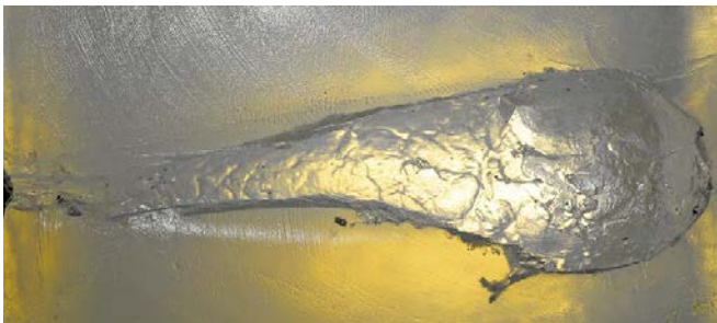
Simulated wound cavity in ballistic soap - .300 Win. Mag. SPEED TIP PRO at 350 m
